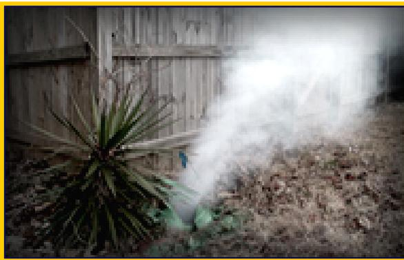
Smoke testing is one of the most efficient and cost effective methods of locating sources of inflow and infiltration problems with sewers.
