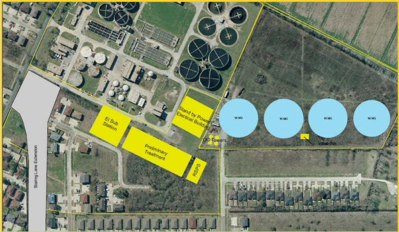
The proposed site layout for the South Wastewater Treatment Plant Wet Weather Improvements Project.
