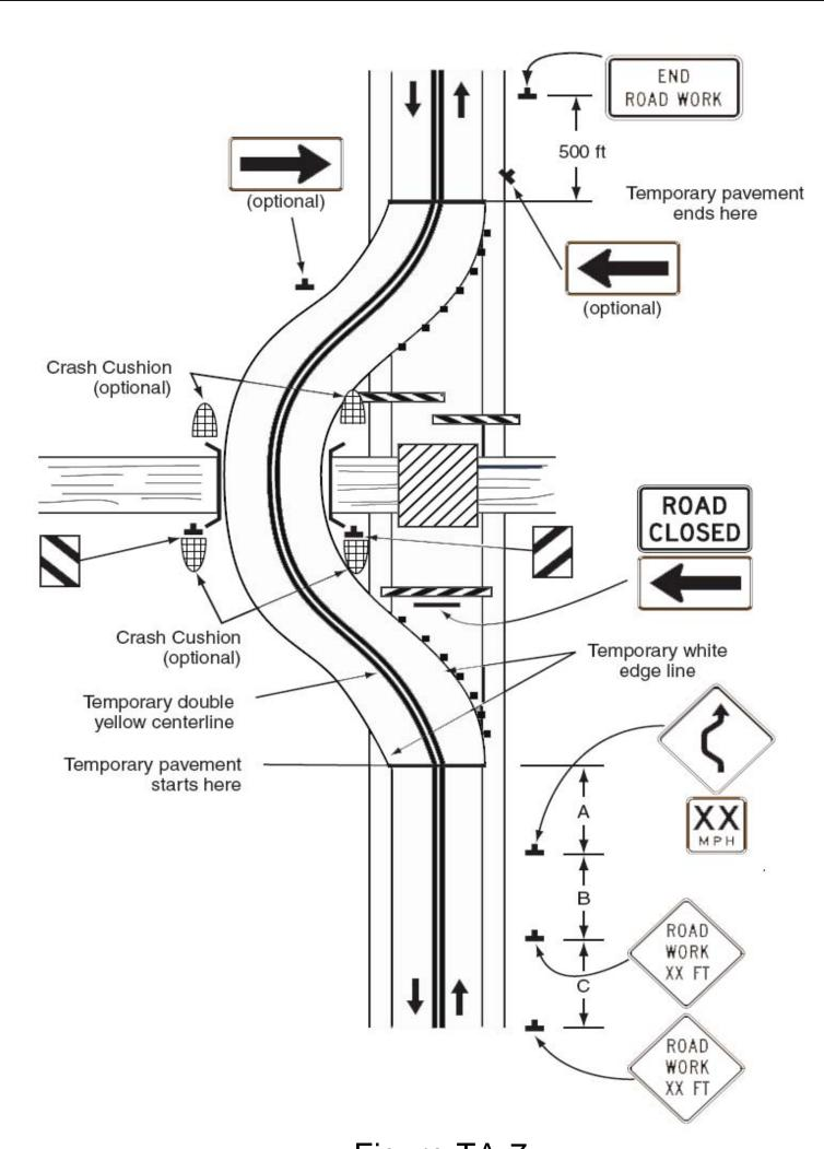
Figure TA-7 Road Closed with Diversion
